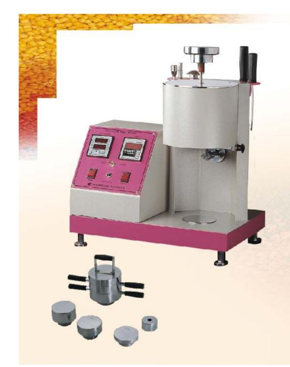
Melt Flow Index Tester as per ASTM D 1238 to measure the flow rates of thermoplastics by extrusion plastometer. This test indicates the uniformity of the flow rate of the polymer.
